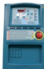
The QAMPE panel permits the control and the management of the generating sets in case of emergency with the main. It controls the main, the engine and the battery and intervenes in case of necessity. It is also provided with a manual command in case of electronic breakdown that keeps active the protections of the generating set. It get ready for remote control and is equipped with a powerful and precise battery charger.
