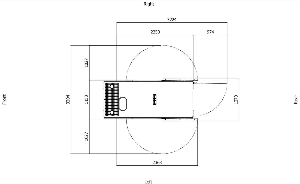
Note: With Lifting-Off Door Solution consider only canopy dimensions.
